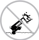
Use extreme care and slow speeds while driving the machine in stowed position across uneven terrain, debris, unstable or slippery surfaces and near holes and drop-offs.
